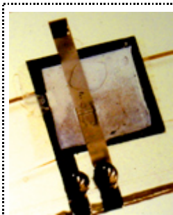
Postage stamp sized research battery that required 140°C to operate
